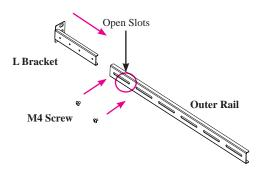
2 Secure L Bracket to outer rail with 1 or 2 M4 screws. Do not tighten yet.
